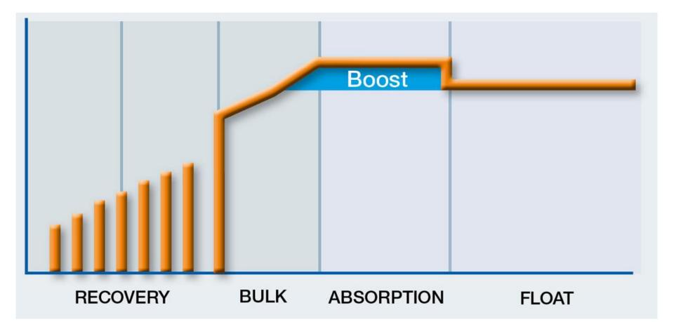
The rapid recovery of almost discharged batteries is guaranteed by the automatic multi-stage charging system (4 charging stages) and the real-time battery diagnostics (8 diagnostic tests).
